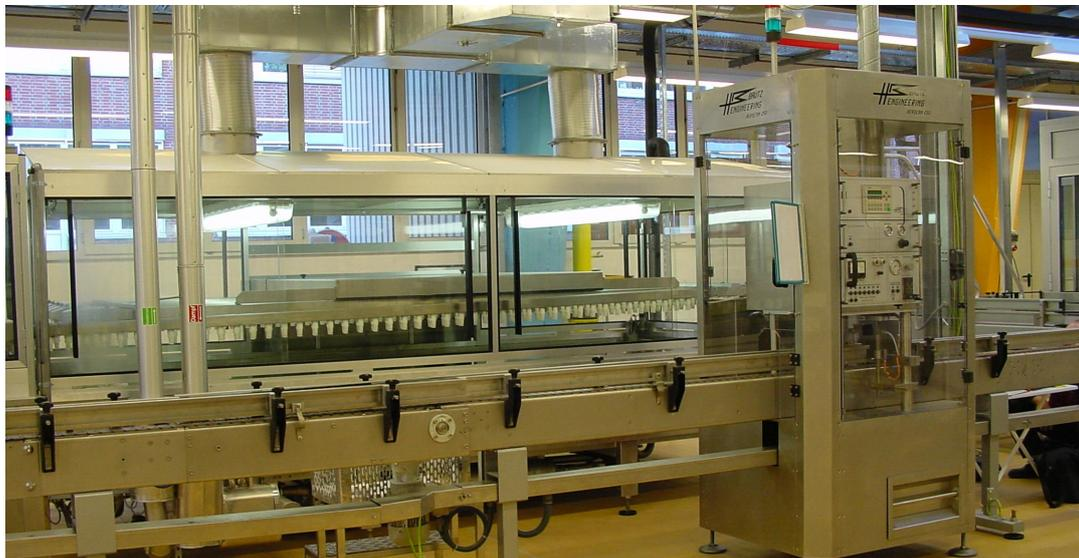
Shown above is our Model AeroCan° 700 leak tester integrated downstream of the water bath. Cans are partially submersed in the hot water bath for burst testing and cleaning.
