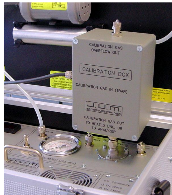
Sample Inlet shown with optional ECB 3000 Calibration Box
